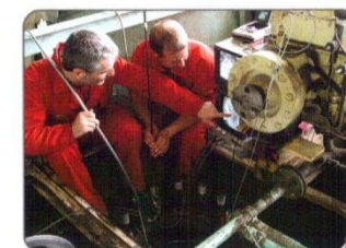
viZaar engineers retrieving penetrant from turbine midstage
